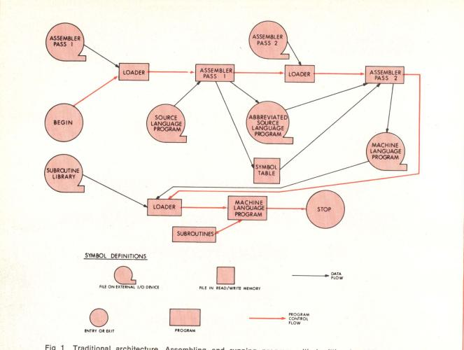
Fig 1 Traditional architecture. Assembling and running program with traditional architecture requires reading in six files and writing two. It is assumed here that loader stays in memory during assembly; otherwise additional reads would be required
