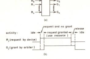
Fig 1 N-channel arbiter resolves conflicts when several devices simultaneously request a shared resource. In (a),  $R_0 \ldots R_n$  are request lines;  $G_0 \ldots G_n$  are grant lines connected to devices  $0, 1 \ldots n$ . In (b), requests are initiated by device upon issuing a ONE signal at its request line. Arbiter allocates resource to device by answering with a ONE signal at corresponding grant line. At a given time, not more than one grant is true
