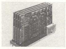
Designated the DR-114, the system is available is 16k x 18 or 32k x 18 configurations and is completely plug-compatible with DEC's MM11-D and -DP single board systems for PDP-11/04 and /34 minicomputers. It has a cycle time of 900 ns and access time of 350 ns. Operating temperature range is 0 to 55°C. Four systems can be combined to provide a maximum capacity of 128k x 18. **Dataram**, Princeton-Hightstown Rd, Cranbury, NJ 08512. Circle 255 on Inquiry Card
