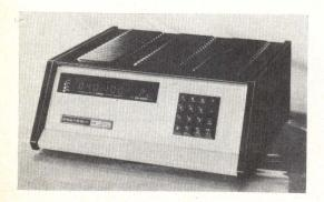
Using the 8080A microprocessor, the Heath H8 is part of a line of hobby, home, educational, and small business computer kits. Computer features an intelligent front panel with octal data entry keyboard and 9-digit, 7-segment display
