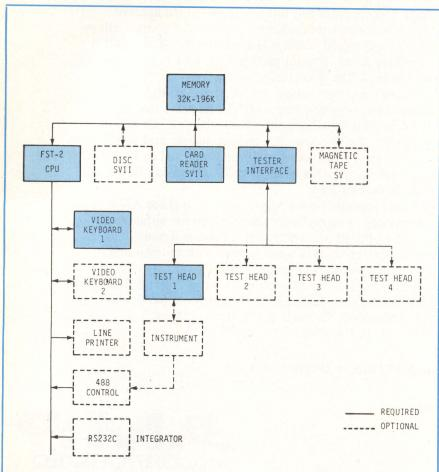
Based on a 24-bit CPU, Fairchild's Sentry V LSI production test system incorporates up to 196k words of semiconductor memory, permitting large increases in test efficiency. Devices handled include microprocessors, peripheral chips, semiconductor memories, and digital hybrids in SOS, ECL, IIL, and other technologies
