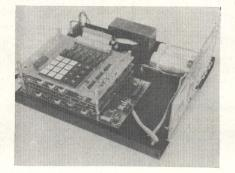
The unit is mounted on a base with its own 5-V switching-regulated power supply. A "blackbox" enclosure allows the unit to be adapted to many industrial and hobby applications. The assembled system sells for \$895.
