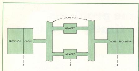
Dual cache bus structure, central to General Automation's shared architecture 16/550 multiprocessor system, connects up to eight processors to a shared memory facility. A single bus can transfer data between four processors and four memory banks at rates of 8M bytes/s
