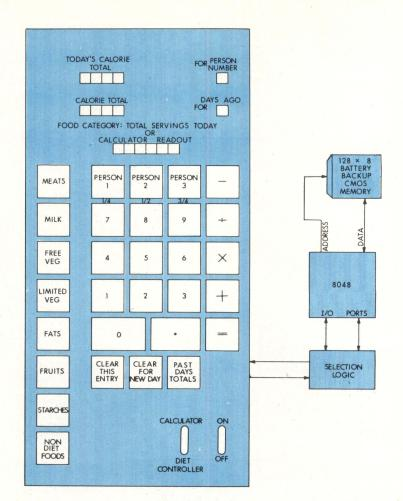
Keyboard design of microprocessor-based controller contains keys necessary to govern diet by accounting for all foods and keeping track of daily and accumulated calorie totals for up to three people. Complete with an 8048 microprocessor and 128 x 8 CMOS memory, device can also be utilized as a calculator
