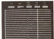
Compare input data with expected pattern in memory and see errors as difference bits.
