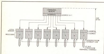
Micral M System can be configured with up to eight microcomputers which operate with separate I/O buses, memories, and interrupt systems, as well as with shared memory
