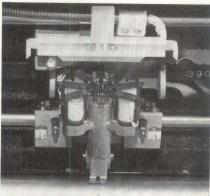
Producing sufficient character density for use in printing bar codes, the Centronics 306 SC incorporates a dot matrix mechanism such as that shown at top. Tally's T-1612 teleprinter incorporates a printhead (bottom) that positions needles and coils for maximum straight line design, because needle wear increases proportionally to curvature
