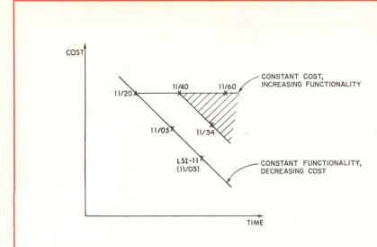
Fig 1 Minicomputer family evolution. Advances in technology translate into two design styles: constant-cost, increasing-functionality and constant-functionality, decreasing-cost. The 11/60 represents former design style. Functionality added to 11/40 is depicted by shaded area. Tradeoffs discussed occur within this area
