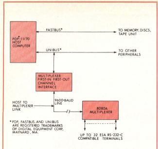
Fig 1 Overall system. Block diagram shows special host computer-to-channel interface: FIFO board and 9600-baud link to 8080A multiplexer. The 32 terminal lines may be any mix of baud rates in groups of four for each rate. Multiplexer may be located in host computer or in its own remote package
