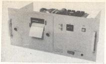
DTL/TTL-compatible is standard. Options include an integral date/clock, paper-low indicator, and event counter. **Master Digital Corp**, 1308-F Logan Ave, Costa Mesa, CA 92626.
