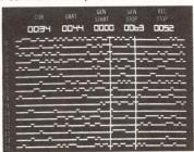
Generate up to 64, 16 bit words parallel so you can test your interfaces.
