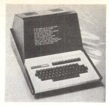
Peripherals, compatible with the two Heath computers as well as others, include the H9 12" (30.48-cm) CRT terminal with 67-key ASCII keyboard and 5 x 7 dot matrix display
