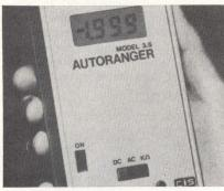
Using low power 31/2 digit LCD plus CMOS logic design, Autoranger operates from a single 9-V battery. Features include total automatic operation with autoranging, autozeroing, and automatic lead reversal. The ac/dc voltage to 1000 V and resistance to 1000 k $\Omega$  are tested with high accuracy and resolution. Portable high impact case has protected switches. **Control & Information Systems, Inc,** 10 Spring Valley Village, Richardson, TX 75080. Circle 263 on Inquiry Card
