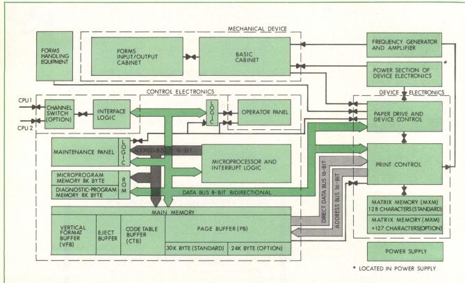
Microprocessor-based control electronics handle data transfer, page buffer loading, and printing system functions of the Siemen's nonimpact ND2 printer. Unit uses laser technology and an electrophotographic printing method to produce 21,000 lines/min on ordinary computer paper
