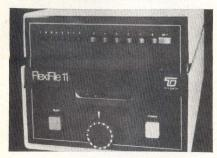
Made up of single- or dual-drives, 8080A microprocessor, and 115-Vac, 60-Hz, 300-W power supply, the FlexiFile 11 is available with optional RS-232 or 8-bit parallel interfaces. Storage capacity is 98k bytes/disc with a transfer rate of 5k bytes/s parallel, 19,200 baud serial. The front panel offers flexibility by means of six mode select switches, and eight indicator lamps which are software defined. **Tri-Data Corp**, 800 Maude Ave, Mountain View, CA 94043.
