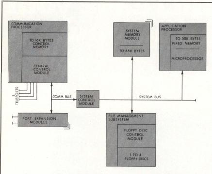
Architecture of Western Union Data Service's Smarts Controller. It contains three functionally-oriented microprocessors for fast response and efficient throughput. Basic system has communications, file management, application, and system memory and control module boards. The last creates data bus and determines which module can access system bus or data path, based on established priority
