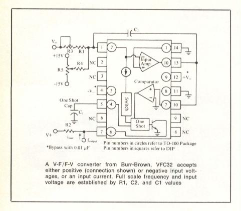
shot capacitor are required for operation. Tempco of the full scale accuracy is ±100 ppm/°C max; input offset voltage drift is ±2 ppm/°C.
