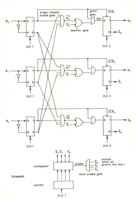
Fig 2 Multichannel arbiter system. Single requests pass through channel and release grant in a direct manner. Multirequest conflict is resolved by scanner that selects channels one at a time. When true scanner output,  $S_k$  ( $k=1\ldots n$ ), coincides with true request signal R, grant  $G_k$  is issued. Irregular request frequency is assumed; at regular frequencies with possible interaction with clock frequency, scanner should be replaced by random number generator
