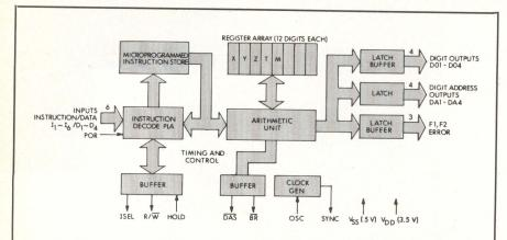
Low power, low cost number cruncher unit from National Semiconductor is preprogrammed microcontroller offering scientific calculator functions. Internal 4-phase clock generator drives unit, which has typical supply current of 12 mA
