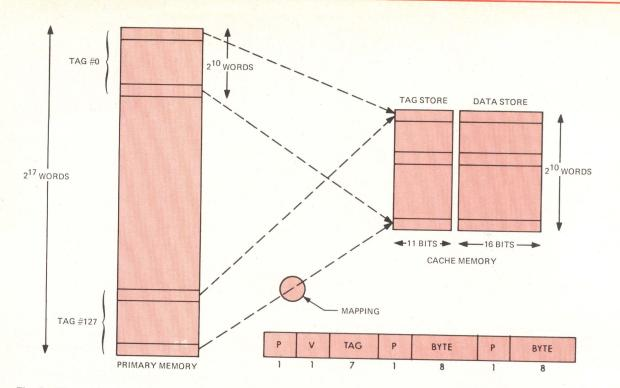
Fig 5 Direct mapped cache. Mapping occurs from 128k words of primary memory to 1024-word cache. High order seven bits of an 18-bit address are stored in tag store to ensure uniqueness in mapping. Tag store also holds a valid bit and parity bits. Cache word format (27 bit in total) is as shown in the
