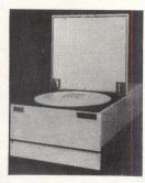
Capacities of 25M, 50M, and 76M bytes of fixed and removable storage are available on the model 312 system. Multiple units can attain a capacity of up to 305M bytes. Data transfer rate is 5 MHz, and average access time is 35 ms. The system is a self-contained random-access storage unit with power supply, logic chassis, and integral clean air mechanism. Options exist for the use of two or three fixed discs plus a re-
