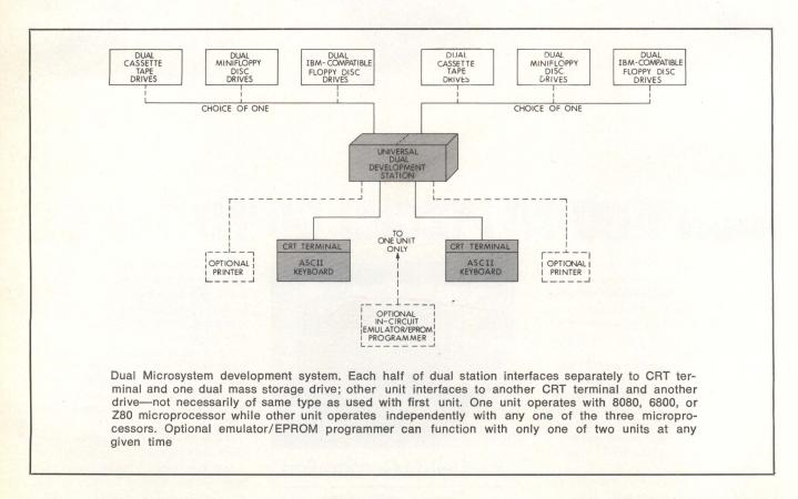
Each unit of the dual configuration contains five I/O channels: CRT interface, keyboard with miniconsole interface, dual tape interface, dual EIA RS-232-C interface, and 8-bit parallel I/o board. All I/o devices have maskable interrupts. The individual system bus is universal, with no card slots assigned to a particular peripheral device, controller, or CPU.
