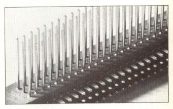
Diallyl Phthalate is the insulator in most models. And all connectors are designed to meet conditions of MIL-C-55302.
